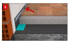
**Installing Fascia Tagliamuro.** Before installing all the partitions, Isolmant Fascia Tagliamuro must be laid. This high density,reticulated polyethylene foam accessory is specifically designed to disjoint partitions and slabs, thereby helping to reduce the structural sound transmission from the walls to the slab. This product is available in different thicknesses and densities depending on the weight of the partitions (Fig.1)
